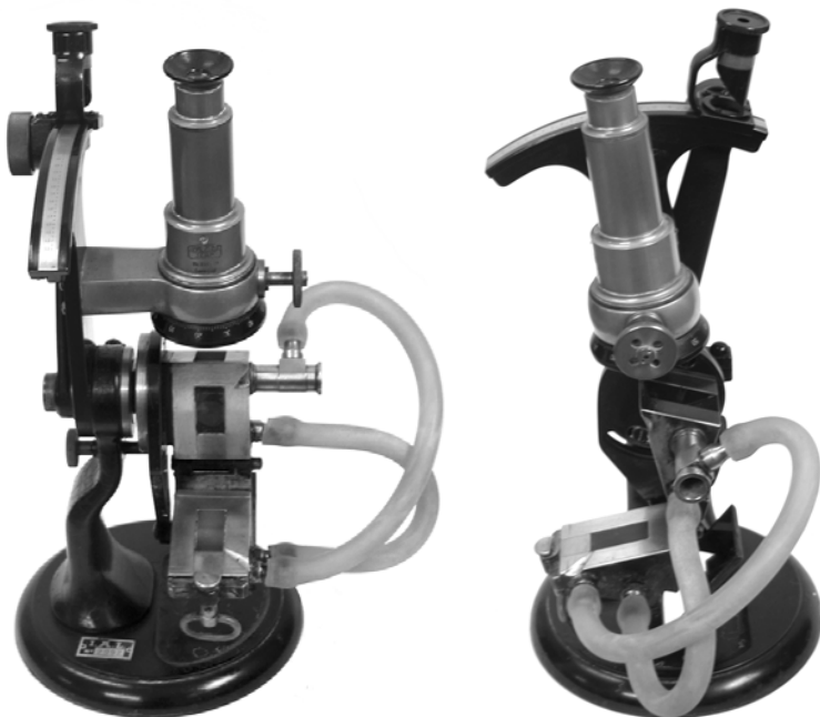
Microscope similar to the one Lutz developed in the 1880s to study protozoans, helminths and insects. It is attached to an apparatus that keeps amoebas warm (Instituto Adolfo Lutz).
